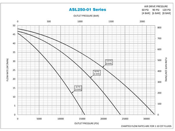
Actual flow rates will vary depending on air flow capacity, downstream flow restrictions, and fluid type.
