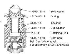
Can be operated by a cam or machine member. Has 3/16" overtravel after full actuation. This valve can be panel mounted. Pressure angle should not exceed 15° from vertical center line. Cam follower is hardened 430F stainless steel.
