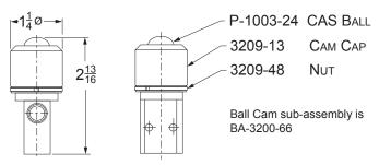
Can be operated by a cam or machine member from any angle, but pressure angle should not exceed 20° from vertical center line. Cam follower is hardened chrome alloy steel.
