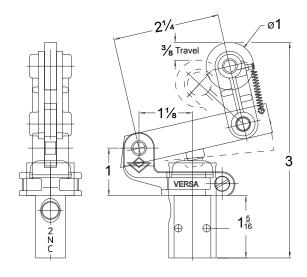
Bracket and Trip-Cam Lever is sub-assembly BA-3200-40-35.
