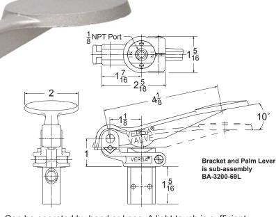
Can be operated by hand or knee. A light touch is sufficient.
