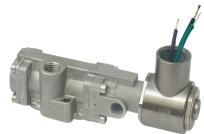
The Versa C316 Series stainless steel NAMUR valve 5-port design can be ordered as either a 4-way for double acting actuators, or as a 3-way for spring return actuators. When the 3-way function is utilized, the unused exhaust port becomes an actuator vent where a filter/muffler can be installed to prevent contaminants from entering either the valve or the
