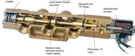
Cutaway shows side-ported "Oil-Free Service" Series "V" . . . one of many models in the complete Versa line.
