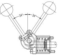
Miscellaneous Single Detent-Spring Center (D – One Direction) Cap Assembly CA-4302-74-111 For ½" Thru ½" Valves This Cap Assembly is denoted in the prefix letters of the valve product no. by the letter
