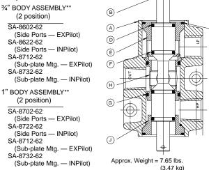
Body Assembly Numbers are for "V" Series valves. For "T" Series, place the letter "T" in front of no. shown: i.e TSA-7202-62.
