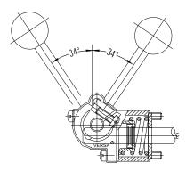
\* Hand-Spring Return (R) Cap Assembly CA-4302-69-130A For ½" Thru ½" Valves
