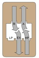
HP inlet open to cylinder port A; cylinder port B open to exhaust
