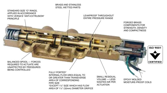
EVERY VALVE FUNCTIONALLY TESTED THROUGHOUT COMPLETE PRESSURE RANGE BEFORE SHIPPING
