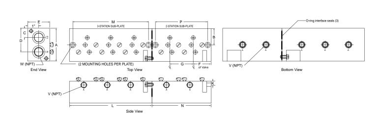
Dotted extension shows detail for 3-Station Co-Ordinate. Pilot Manifold Adapter plates are available for mounting pilot valves with manifold mounted pilot ports. Consult factory.
